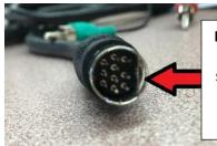
**Note**: Arrow to Arrow. Arrow on the cable connector that must match up to the Arrow on the box. Make sure flat spot lines up. **Important**: If not matched up correctly the pins bend/break easily and the box it will not work.
