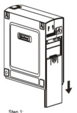
Slide off the battery cover at the back of the
