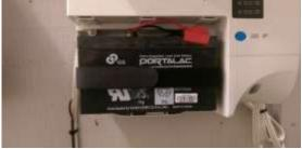
Finally, replace the battery compartment cover. Plug the power supply back in to electrical outlet. The Missing Battery and Replace Battery lights should now go out within 15 minutes.
